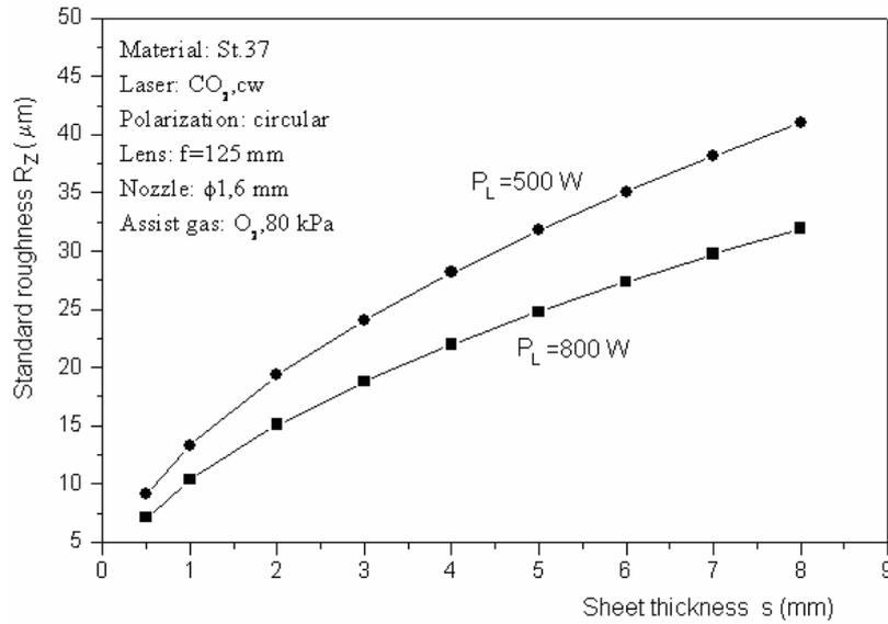
Fig. 4. Surface roughness in dependence of sheet thickness.
