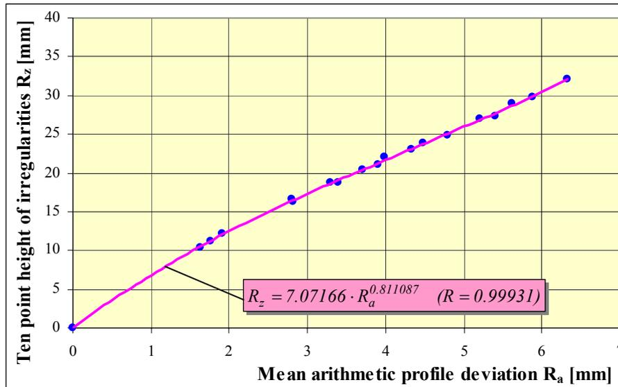
Fig. 6. The ten point height of irregularities  $R_z$  versus mean arithmetic profile deviation  $R_a$  for exponential mathematical model.
