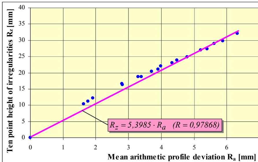
Fig. 5. The ten point height of irregularities  $R_z$  versus mean arithmetic profile deviation  $R_a$  for linear mathematical model.
