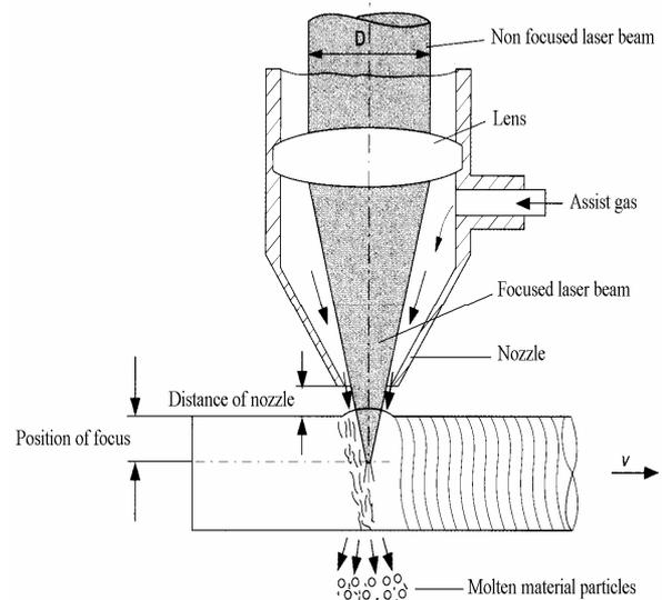
**Fig. 1.** Gas assisting laser cutting.
